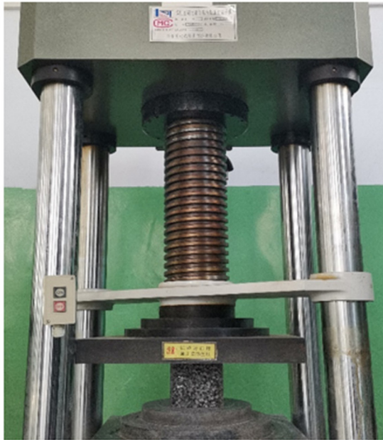
Figure 1: Microcomputer-controlled electro under-hydraulic servo hydraulic press.
