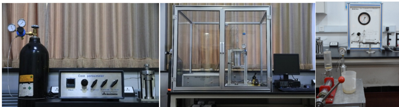
Figure 3: Pictures of PDP permeability tester, steady state permeability tester, and porosity tester.
