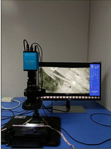
Figure 6: Characterization by high-definition CCD optical microscopy.
