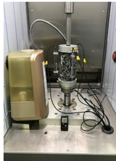
Figure 5: Schematic diagram of the DTS dynamic modulus test.
