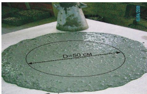
Figure 3: Determination of the flowing time of the mixture (slump flow time, T_{500} , s).
