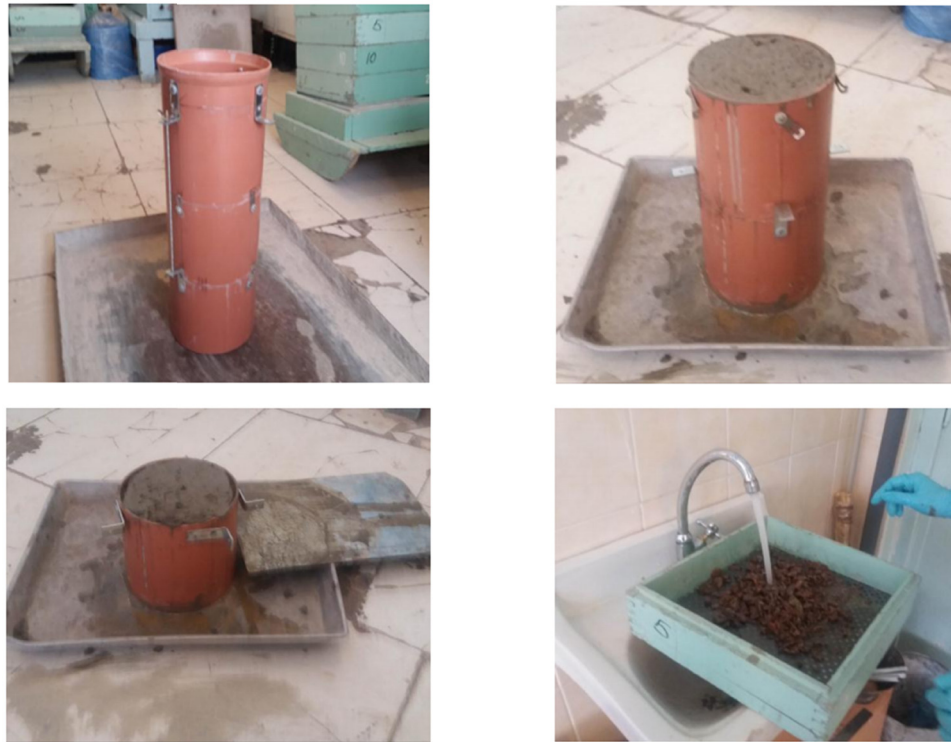
Figure 4: Determination of SCC resistance to segregation in a three-section cylinder.
