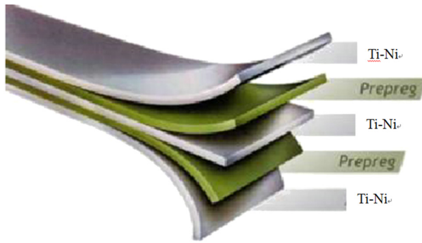
Figure 4: Lamination of pipelines.
