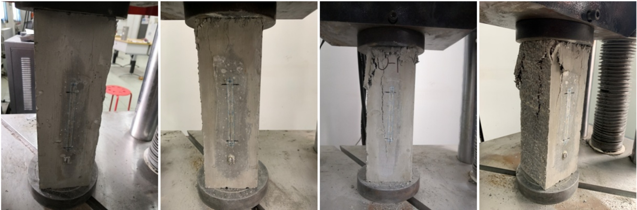
Figure 7: Failure mode of group U specimens.
