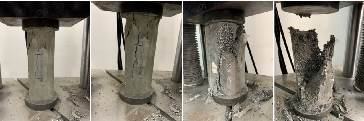
Figure 6: Failure mode of group M specimens.
