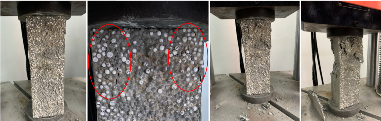
Figure 5: Failure mode of group Y specimens.
