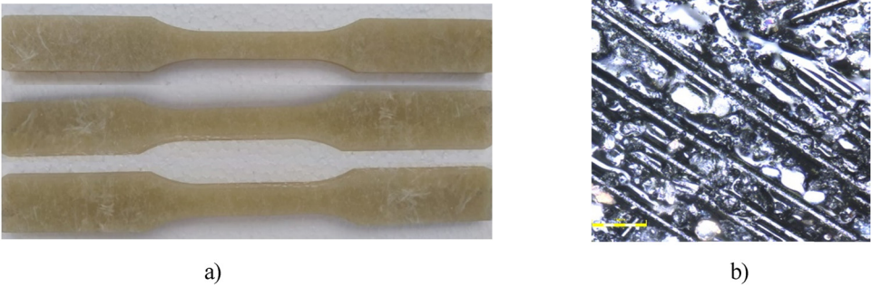
Figure 5: View of samples with 10% recycle content (a) and structure of the K10 composite at magnification 50× (b).
