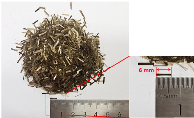
Figure 1: Morphology of 6 mm long basalt fibers.
