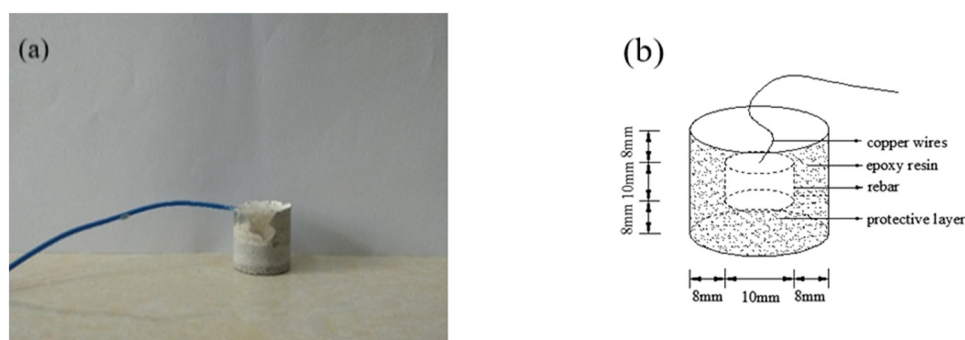
Figure 1: (a) Electrochemical specimen and (b) electrochemical impedance spectroscopy specimen model.
