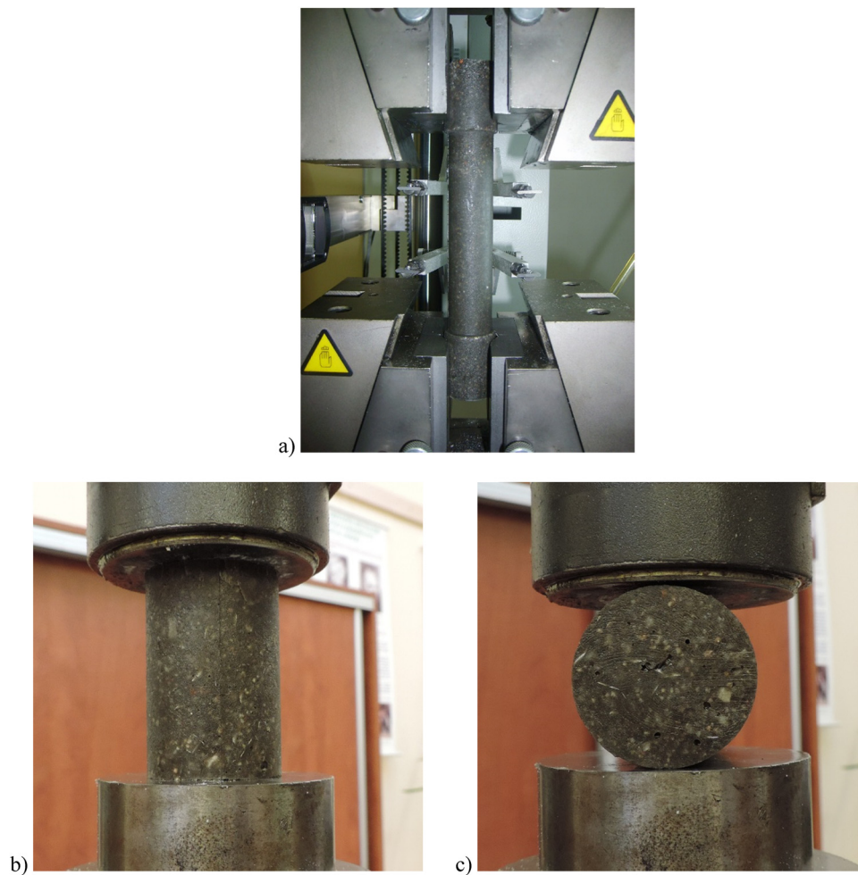
Figure 2: Views of specimens mounted in measuring apparatus (a) for tensile strength, (b) for compressive strength, (c) for splitting tensile strength.
