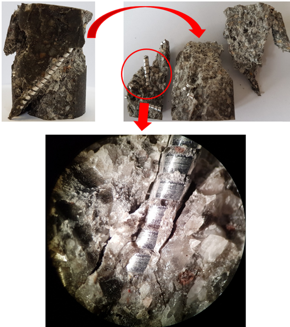
Figure 10: Example of fracture of the specimen after the test.
