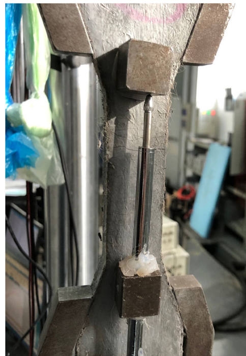
Figure 4: Uniaxial tensile testing set-up and specimen with LVDT.
