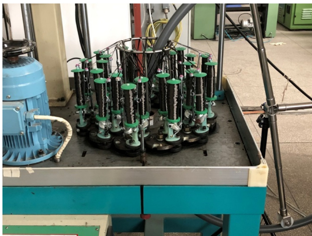
Figure 2: Actual image of the annular axis braiding machine.
