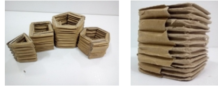
Figure 4: Deformation mode of paper corrugation tube along X direction
