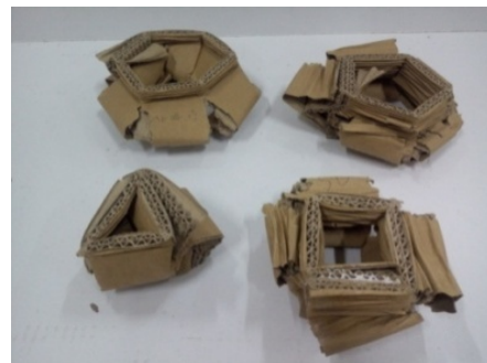
Figure 5: Deformation modes of paper corrugation tubes along Y direction
