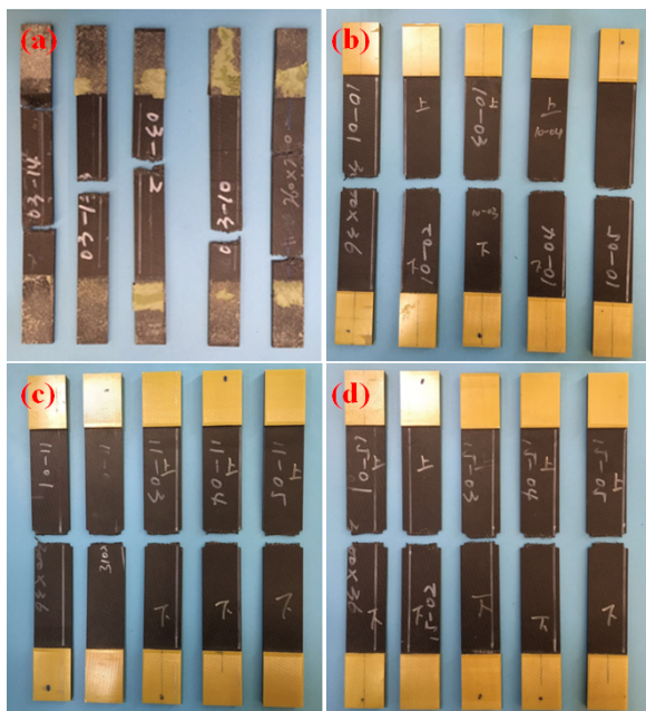
Figure 4: View of specimens after tensile test (a) No damage (b) 2mm depth of notch (c) 3mm depth of notch (d) 4mm depth of notch
