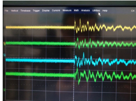
Figure 4: Waveforms of signals collected by strain gauges
