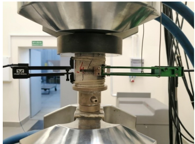
Figure 5: One of the samples of adhesive mortar with the extensometers for measurement of deformation during the compressive strength test.
