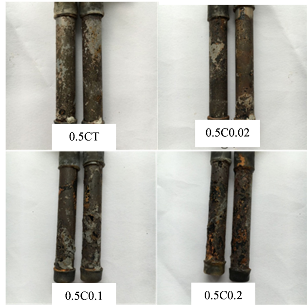
Figure 10: Corrosion condition of reinforcement
