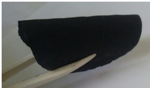
Figure 6: Photograph showing the elasticity of the three-phase conducting polymer nanocomposite.
