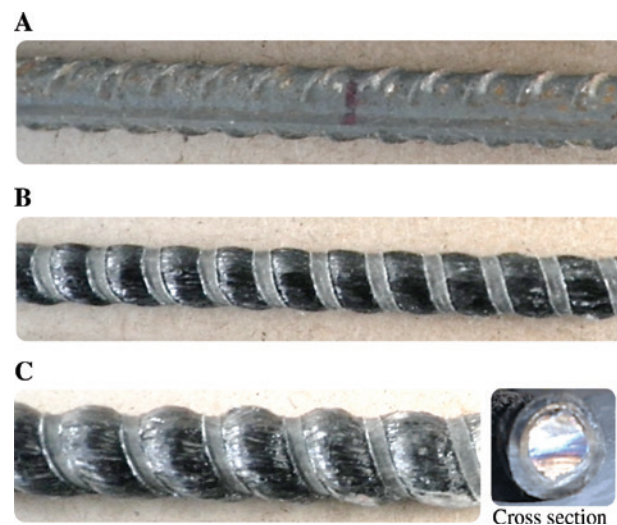
Figure 1: Longitudinal reinforcing bars in this study. (A) Steel bar, (B) BFRP bar and (C) SFCB.
