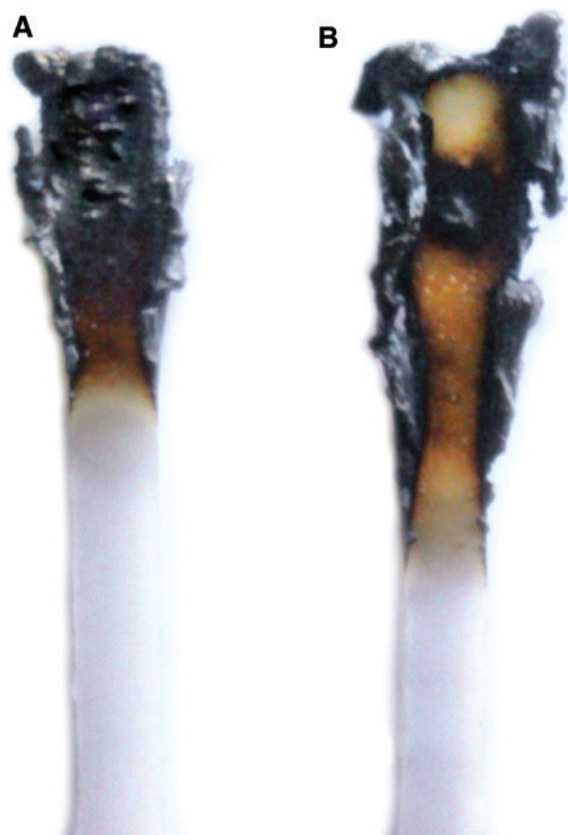
Figure 2: The char residue in: (A) 20APP and (B) 15APP5AG.
