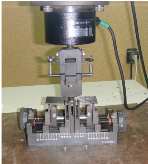
Figure 11 End-notched flexure (ENF) specimen for mode II testing mounted in the fixture.
