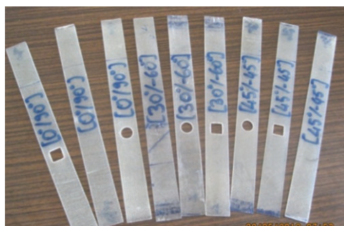
Figure 2 Laminated glass-polyester composite plates.
