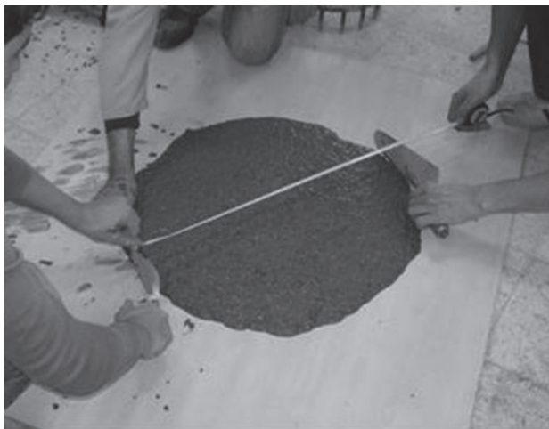
Figure 2 Measuring of flow diameter of SCC and SCLC after slump flow test.
