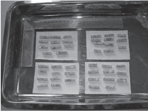
Figure 4 Prepared specimens for thermal expansion measurements.
