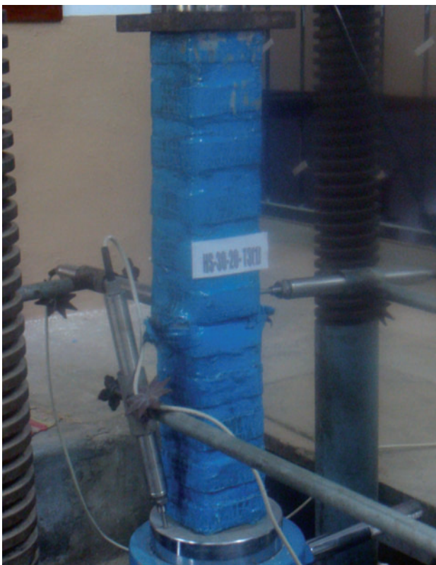
Figure 8 Failure mode of HS-30-20-T3.
