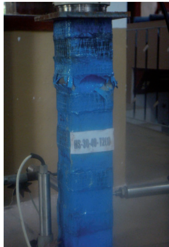
Figure 10 Failure mode of HS-30-40-T2.
