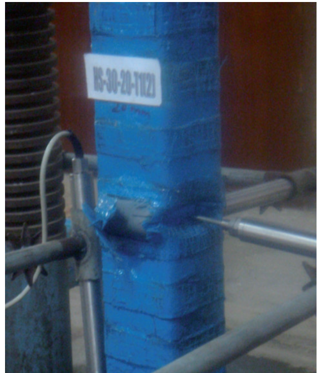
Figure 6 Failure mode of HS-30-20-T1.
