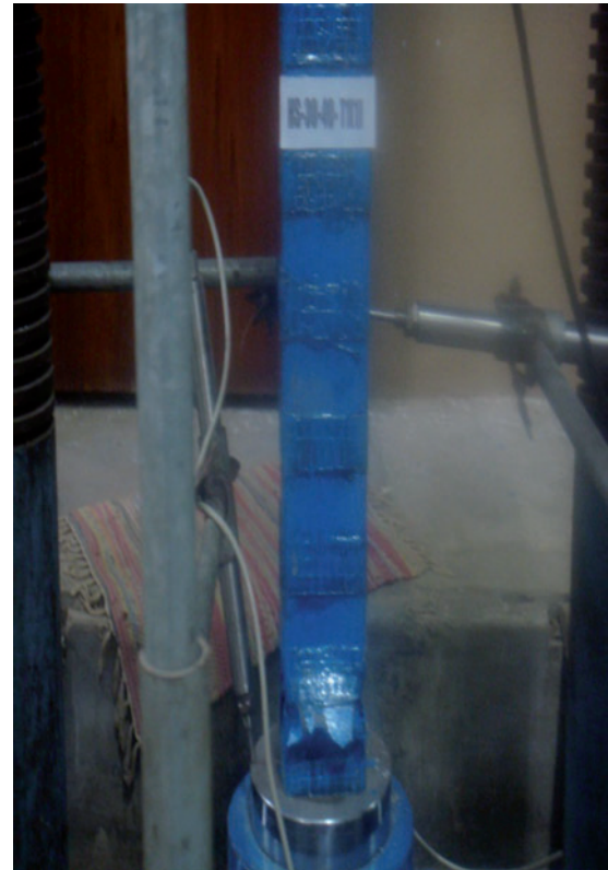
Figure 9 Failure mode of HS-30-40-T1.
