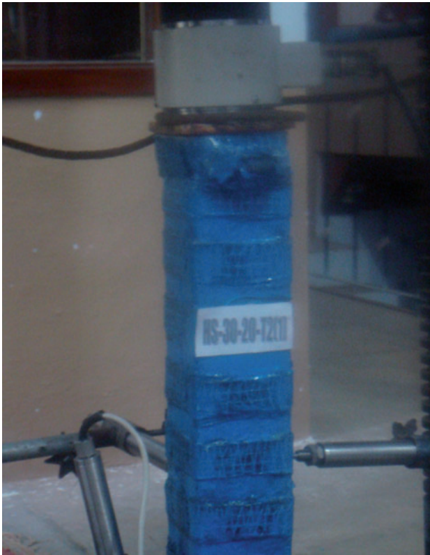
Figure 7 Failure mode of HS-30-20-T2.
