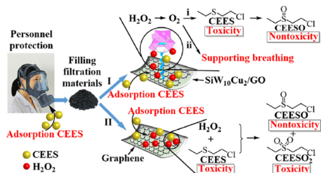
Figure 9: The schematic diagram of simultaneous dismutation of \text{H}_2\text{O}_2 to \text{O}_2 and oxidation of CEES by \text{SiW}_{10}\text{Cu}_2/\text{GO} catalyst. Reproduced with permission from ref. 71. Copyright 2020 American chemical Society.
