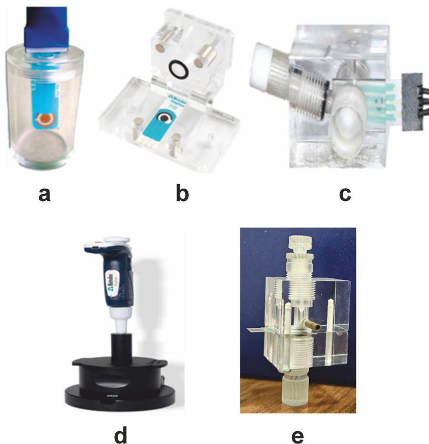
Figure 6: Images of factory-made electrochemical cells for voltammetric analysis using screen-printed electrodes. a) is a stationary mode cell, b) is a DropSens flow-injection cell, c) is a RuSens flow-injection cell, d) batch-injection cell of \Omega metrohm, e) batch-injection cell (this work).
