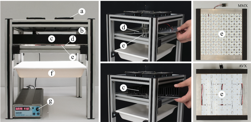
Figure 7: Light bleaching test device with (a) cooling fan, inserted in (b) corrugated cardboard, (c) heatsink, attached to (d) aluminium plate supporting the (e) LED module (here: AVX). The distance between the LED and the tray (f) is adjustable between 3–30 cm. The DC power supply (g) serves as an on-off control and determines the illuminance by setting the desired voltage.
