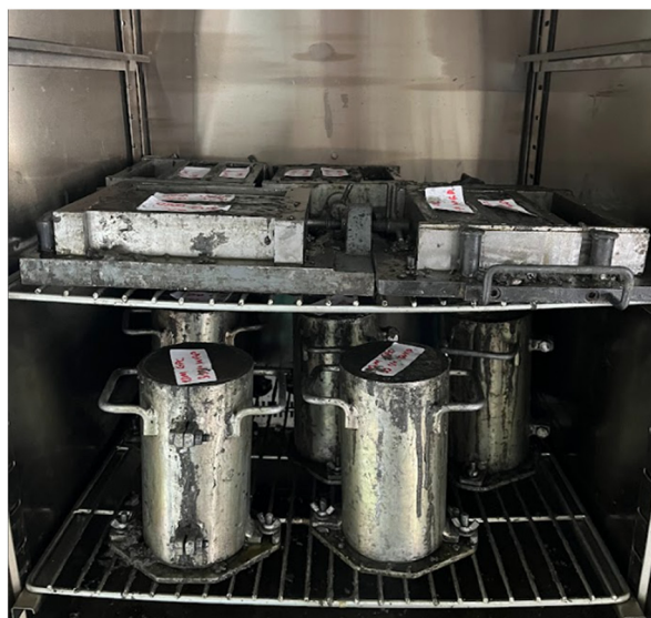
Figure 3: Curing of GPC samples and weight control.
