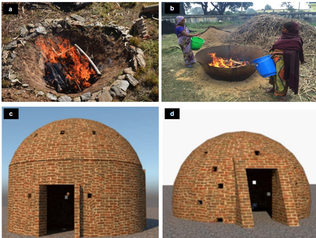
Figure 3: (a) Conical soil pit [84], (b) steel-shielded soil pit [84], (c) Brazilian beehive kiln [77], and (d) Argentinian half-orange kiln [77].
