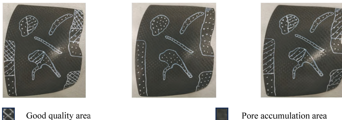
Figure 2: Schematic diagram of abnormal area identification of samples at different frequencies [20].
