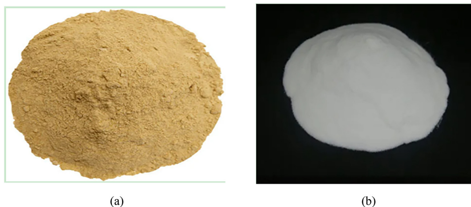
Figure 1: (a) shows Pure PSP, and (b) presents Pure PES samples. Both samples were processed by passing through a 100-mesh screen, resulting in a particle size of 125 \mu\text{m} .
