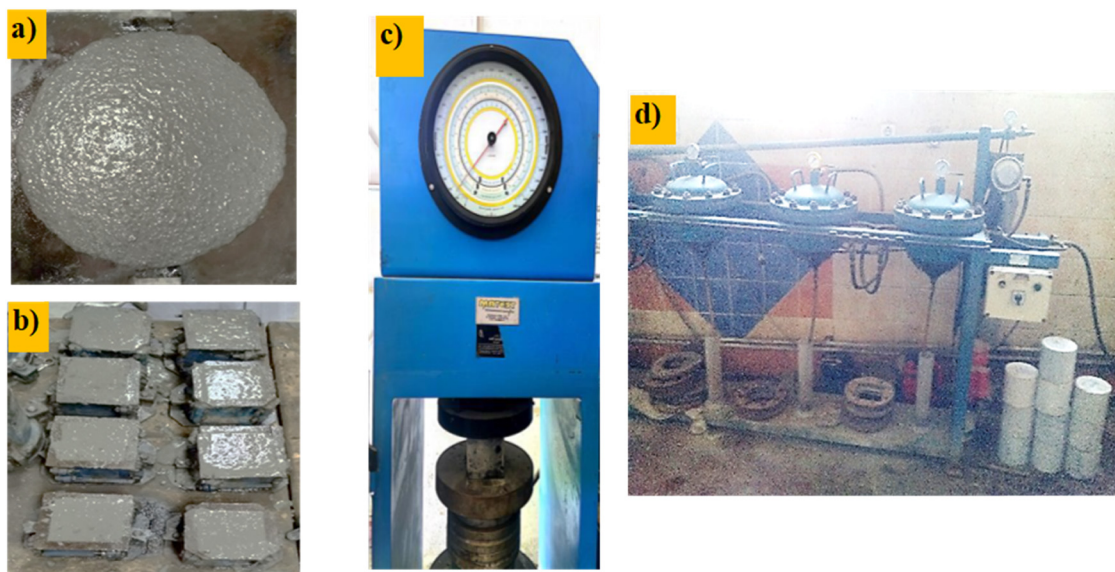
Figure 3: Testing procedure in this study: (a) slump flow test, (b) concrete samples, (c) compression test, and (d) WP.
