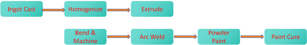
Figure 11: Manufacturing sequence of aluminum extrusions for sports applications.
