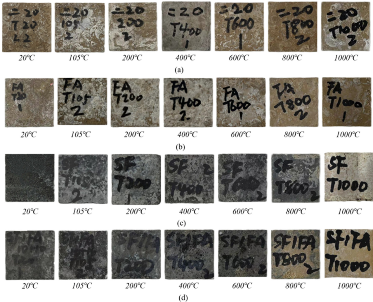
Figure 4: Apparent characteristics of MPC after being treated at different temperatures. (a) M0, (b) F2, (c) S4, and (d) C2.
