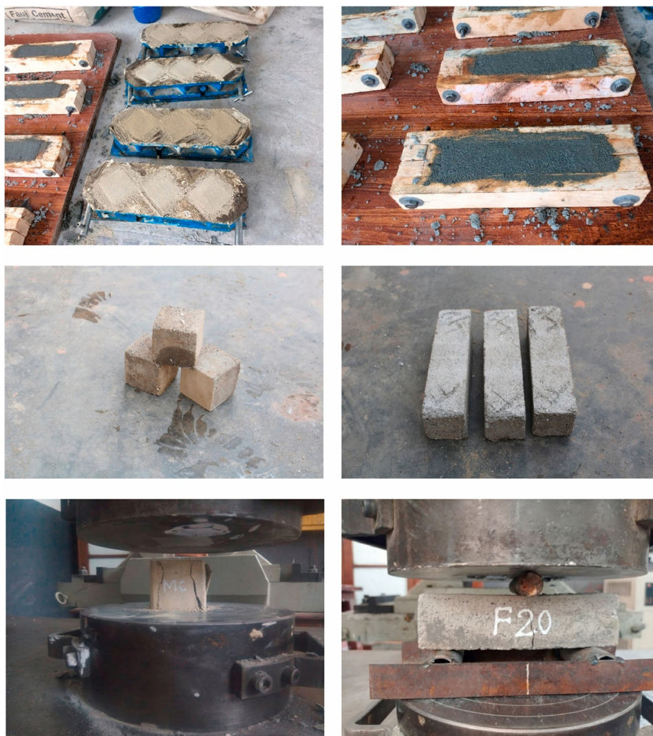
Figure 2: Images of specimens for CS and FS within molds, dried, and during testing [15].
