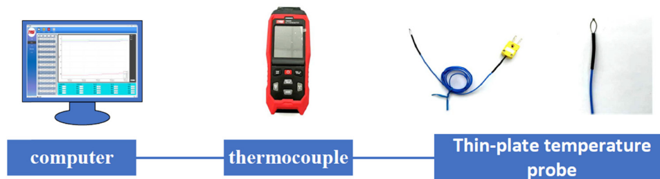
Figure 6: Ramp-up test connection.
