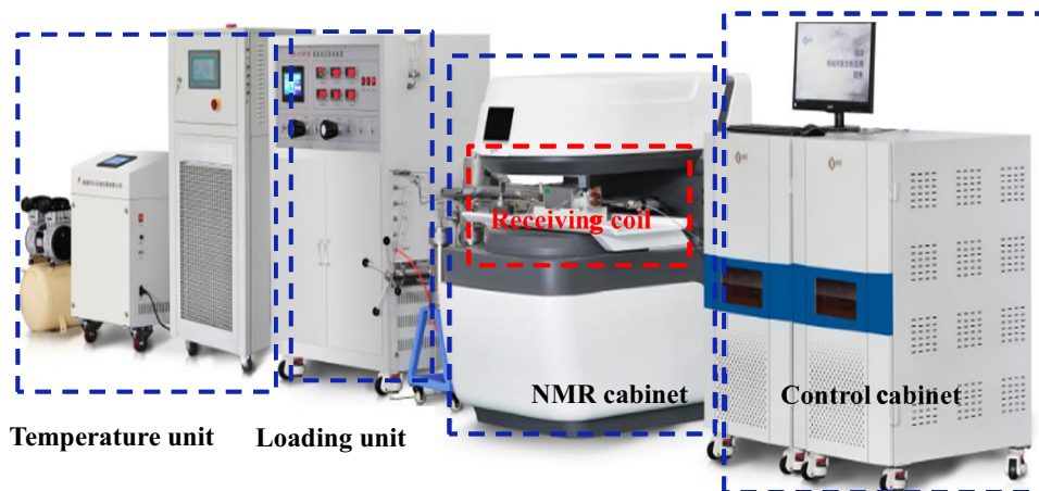
Figure 2: NMR test system (model, MacroMR12-150H-I).
