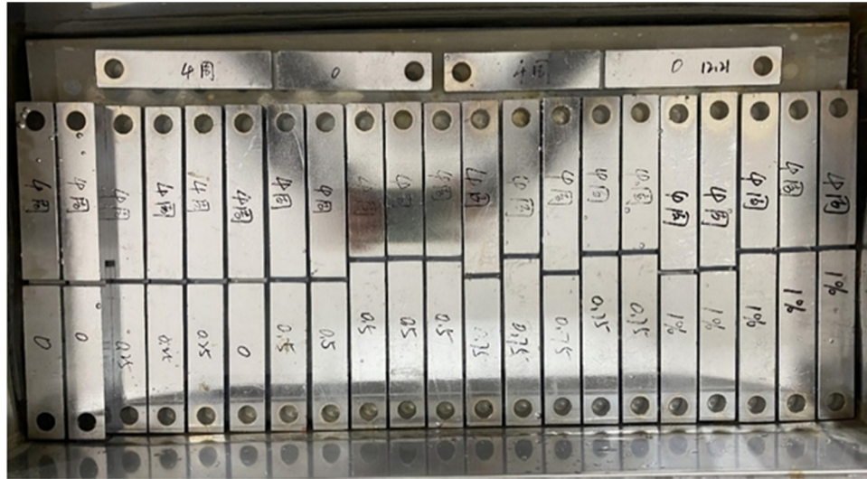
Figure 3: TAST specimens immersed in distilled water.
