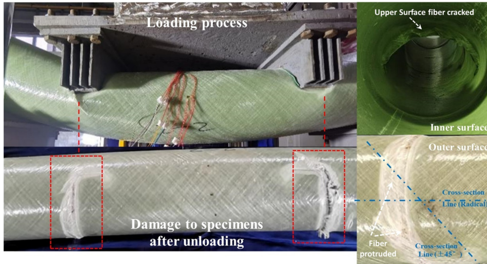
Figure 5: Damage details of specimen F-D320-45.
