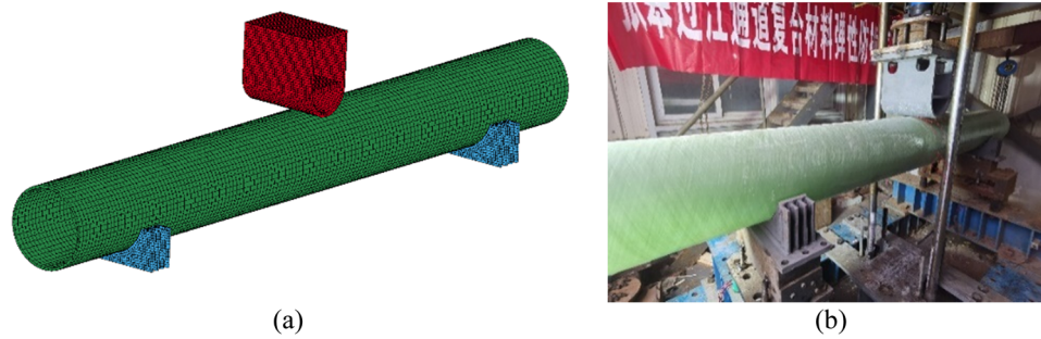
Figure 12: The diagram of vertical impact test and FE: (a) FE models and (b) vertical impact test.
