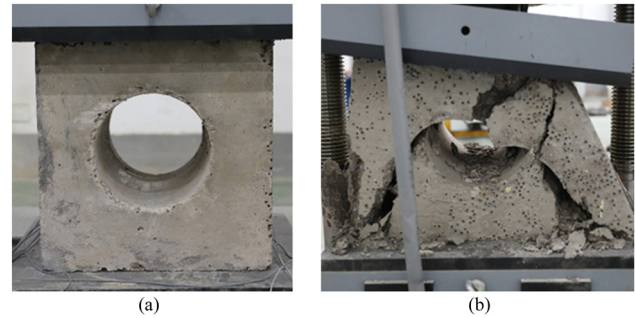
Figure 24: SAP concrete damage state. (a) Initial form and (b) after destruction.
