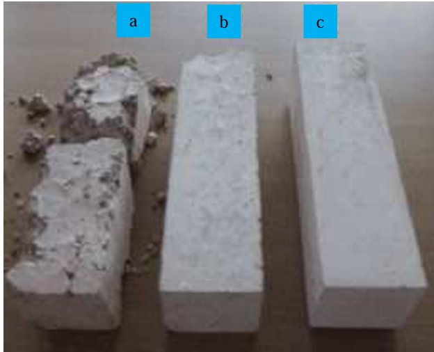
Figure 19: Deterioration of the sample exposed to 30 days at elevated temperature: (a) gravel aggregate, (b) granite aggregate, and (c) ceramic aggregate [80].
