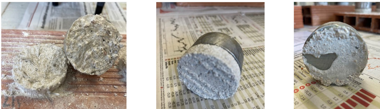
Figure 7: Failure of specimens in adhesive strength test.
