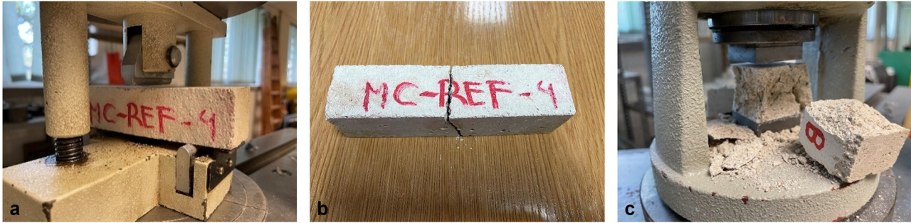
Figure 9: Failure of specimens in mechanical tests (a) flexural strength and (b) compressive strength.
