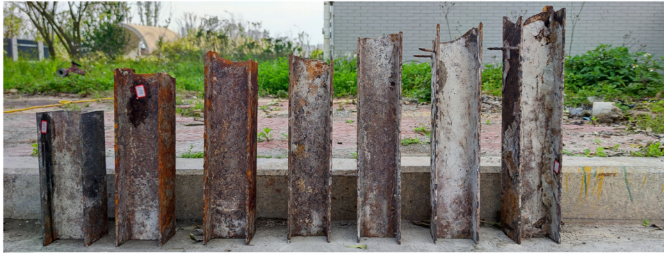
Figure 15: Corrosion of section steel.
