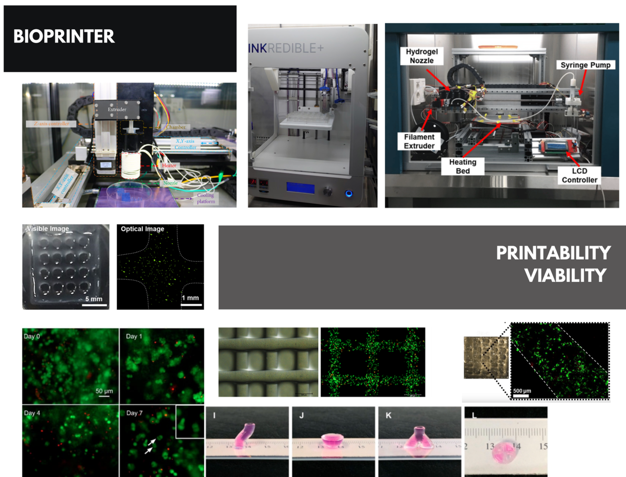
Figure 10: Presentation of commercial and custom-made bioprinters and comparison of printability and viability of bio-ink-embedded cells [57,119,135,140,141], CC-BY license.
