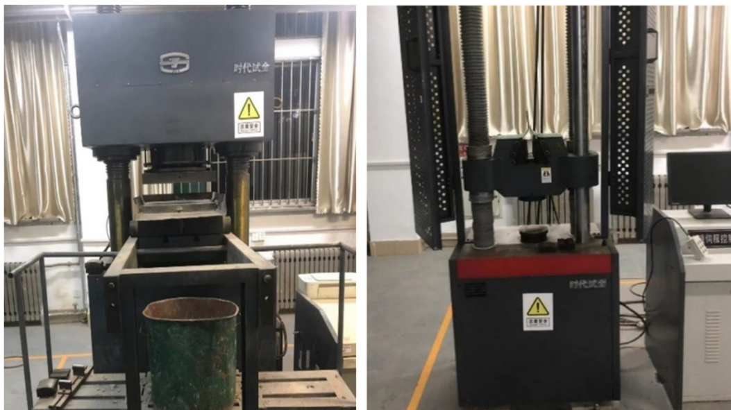
Figure 5: Electrohydraulic servo pressure testing machine.
