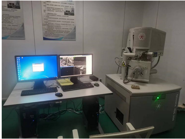
Figure 6: Field emission environmental scanning electron microscopy.
