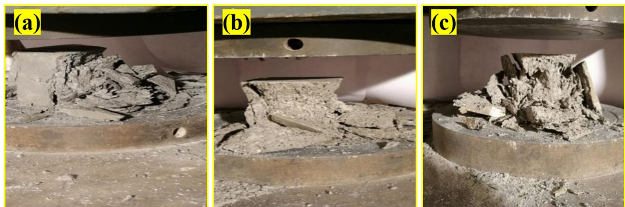
Figure 5: Failure modes of MS-GPM under different ratios of MS to MK and FA: (a) = 1; (b) = 3; (c) = 5.
