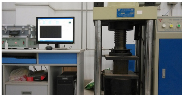
Figure 2: Compressive strength test of a 150 mm cube CSG specimen.
