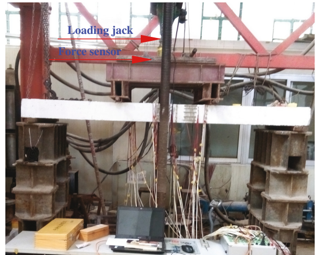
Figure 6: Photograph of the actual loading.
