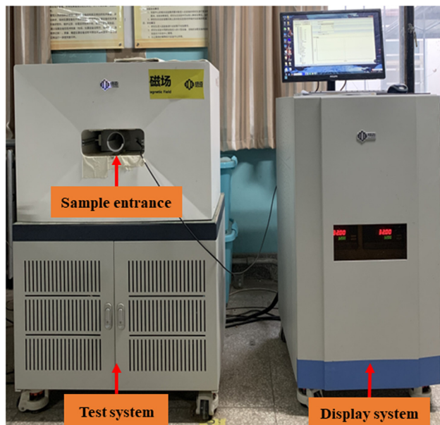
Figure 2: NMR test equipment.
